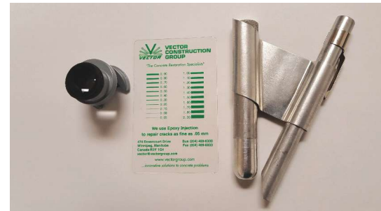
Crack widths can be visually measured using a gauge card (middle) or pocket microscopes. All Photos: Vector Construction.
